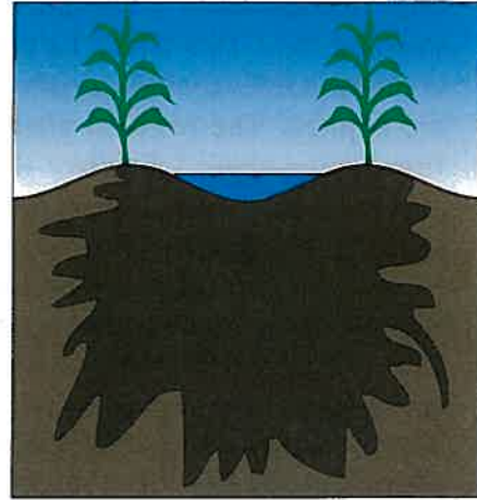
Figure C-4. The wetting pattern under furrow irrigation may be deep and uneven especially during the first irrigation.
