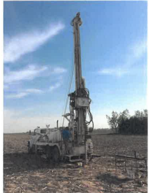
Figure 14 – Geoprobe® (left) and Rotary Drill Rig (right) Used in Vadose Zone Sampling
