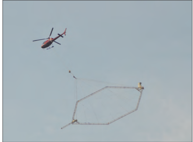
Airborne electromagnetic (AEM) flight over LPSNRD
